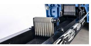
The new dobby drive with increased transmission capacity and the new shedding motion, optimized in combination with the latest dobby model, ensure minimal vibrations of heald frames, with increased warp efficiency ay top speed.
