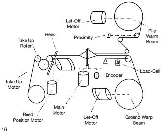
Precision of the electronic let-off motion, stability and repeatability of the warp tension parameters are granted by high accuracy load cell with "self-learning utilities" which ensure excellent fabric quality with
