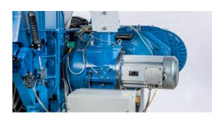
The new sturdy and high torque drive for Jacquard ensures the top running regularity and speed, also in combination with the largest Jumbo Jacquard machines.
