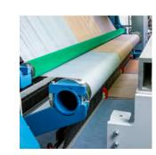
The new PTE - Pile Tension Equalizer system, ensures the gentlest treatment of warp yarns, for a first-rate terry quality, guaranteeing the highest performances also with single-ply and low torsion pile yarn, for the most soft, absorbent and luxurious terry fabrics.
